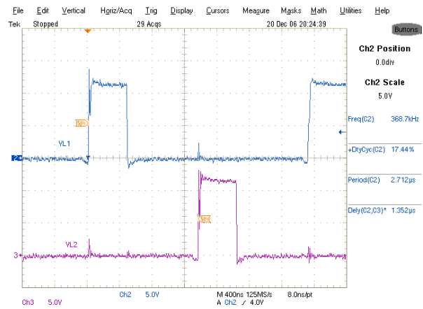
Fig. 32: Inductor points at 60A load.
